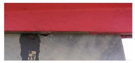
During this operation the centreboard was moved sufficiently to allow a visual check inside the centreboard case. A bulge could be seen on the starboard side.
