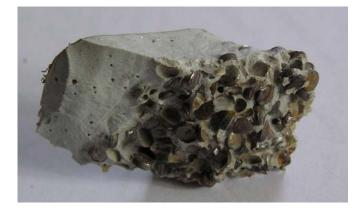
In order to understand my train of thought it is necessary to note that when sailing to windward the centreboard exerts large forces on the centreboard case (especially in strong winds). These forces may be sufficient to cause a crack to form between the fibre glass wall of the centreboard case and the ballast. Once such a crack has formed it provides access to sea water and oxygen. This allows the steel pressings to start to rust.
