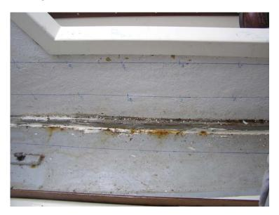
I discovered from discussion with Cornish Crabbers Ltd (now Select Yachts) that the ballast is made up of steel pressings set in a compound of slate dust and polyester resin. In BC each pressing is about 3 mm diameter and 1 mm thick. Several million of these pressings are used to make up the volume of ballast
